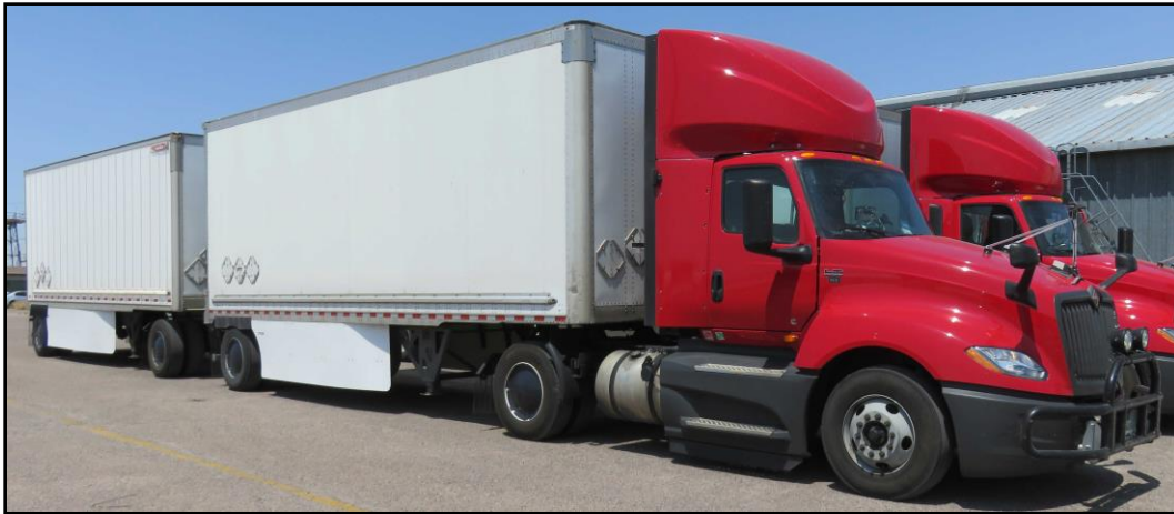
Figure 7: Run 8 Test Vehicle Config. (Eco Flaps and Eco Caps, Truck and Trailer)
