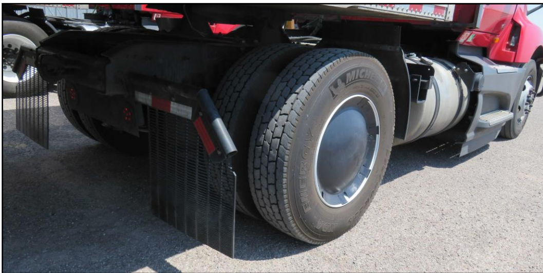
Figure 8: Tractor with Eco Flaps and Eco Caps
