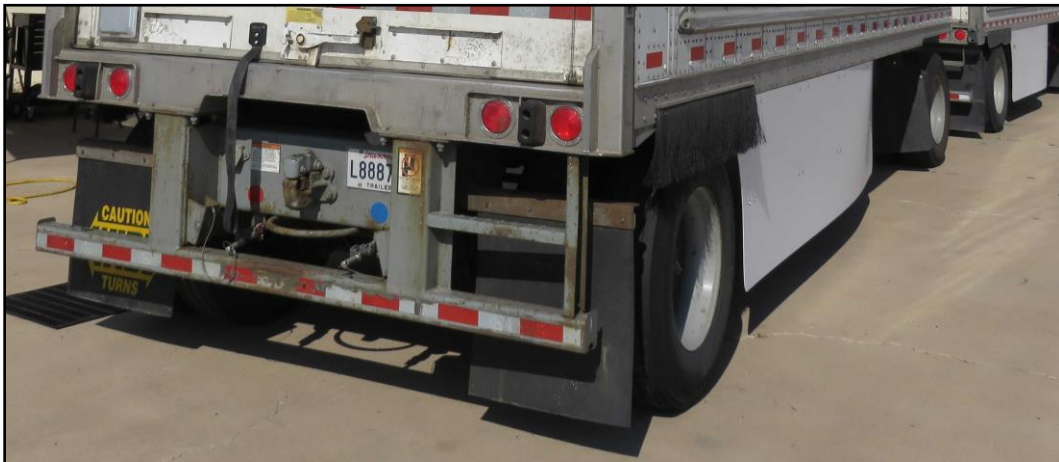
Figure 4: Baseline Trailer (Solid Mud Flaps, No Wheel Caps)
