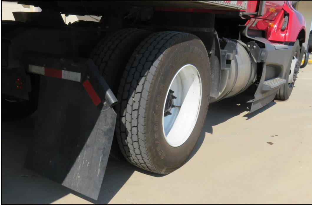
Figure 3: Baseline Truck (Solid Mud Flaps, No Wheel Caps)
