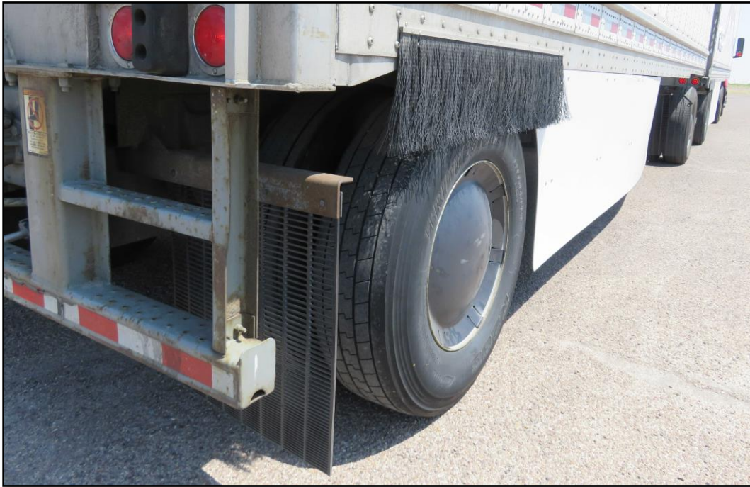
Figure 9: Trailer with Eco Flaps and Eco Caps
