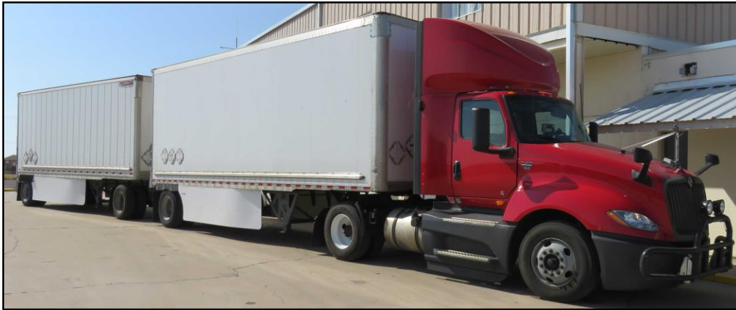
Figure 1: Test Vehicle where Eco Flap Technologies were Installed
